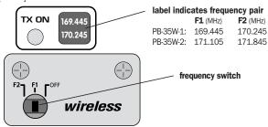
1. Set the frequency of the receiver to either of the two channels, F1 or F2.
